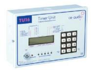
The TU-16 is a versatile 24 hour or 7 day, 5 channel Timer Unit. With the ability to store up to 16 separate events per day, it is capable of controlling a wide range of different external equipment (such as digital message stores and tone generators) via its five individually addressed, fully isolated relay outputs.
